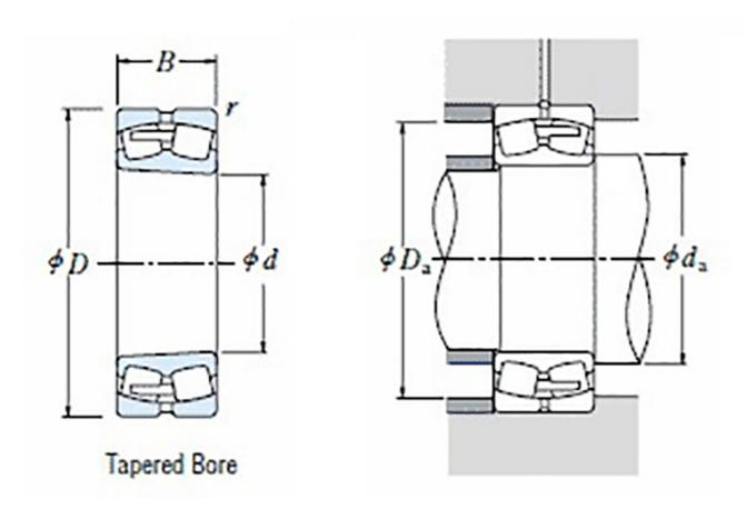
High quality spherical roller bearing with tapered bore from TIMKEN, a world leader in roller bearing technology. TIMKEN spherical roller bearings feature high class materials, innovative cage designs, enhanced surface finishes allowing better lubricant distribution and higher loadratings leading upp to lower operating temperatures and longer service life
